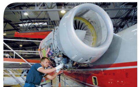
Pratt & Whitney Canada engines, such as the PW305 shown here, are maintained by the CSC in Ludwigsfelde.
